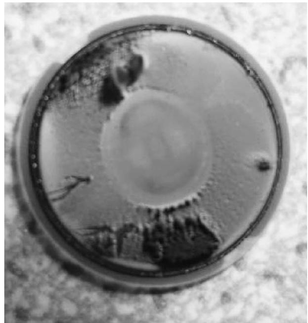
Fig. 4. A 6 MHz plano-convex, AT-cut quartz resonator coated with carbon-nanoparticles while the crystal current was 140 mA.
