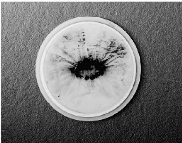
Fig. 3. A 6 MHz plano-convex AT-cut quartz resonator coated with carbon-nanoparticles for 40 min, while the crystal current was 90 mA.
