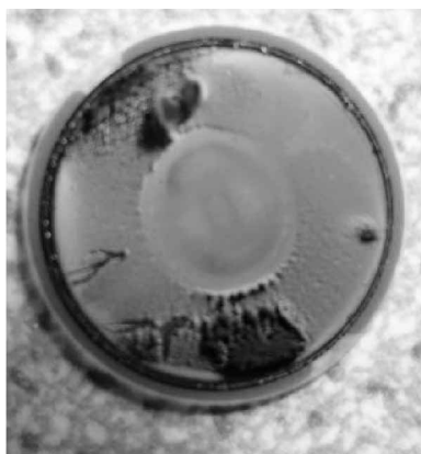
Figure 5. A 6MHz plano-convex, AT-cut quartz resonator coated with carbon-nanoparticles while the crystal current was 140 mA.
